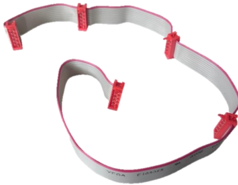
Figure 11: PoExtension2 cable for connecting PoStep drivers with PoKeys57CNC device
